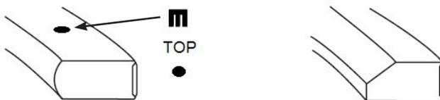
**2nd Ring:** If there is a dot (pip mark) or a laser etching (commonly etched as "TOP" or the MAHLE logo, or a number designator) on one of the flats of the top ring, this marking is indicating the top of the ring. Typically, if there is a bevel on the ID of the 2nd ring, the bevel should be facing down toward the bottom of the piston. Any marking indicating the top of the piston ring supersedes the location of the ID bevel of the ring.
